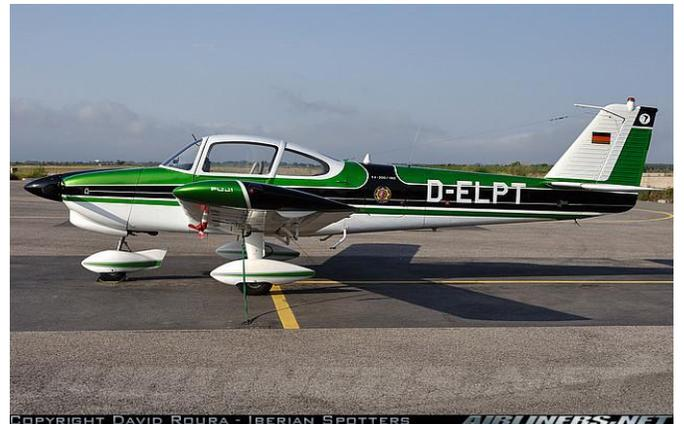
**Fuji FA-200 Aero Subaru:** Built by Fuji Heavy industries in Japan. Development began in 1964. The first prototype flew in August 1965. It is a low wing, all-metal
