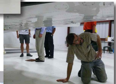
John H, A&P by trade, checking out the Cessna for corrosion ...
